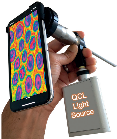
Figure 2. Concept image rendered by the author of a miniaturised portable Quantum Cascade LASER for diagnosing cancer in the larynx when attached to a smart phone endoscope.
