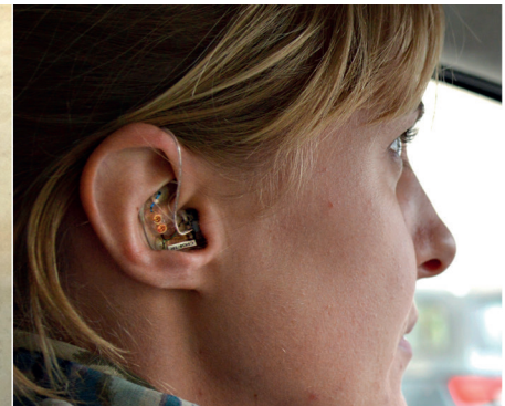
Examples of in-ear EEG mounts. ©2016 Mikkelsen.kaare, CC BY-SA 4.0, via Wikimedia Commons https://commons.wikimedia.org/wiki/File:Ear-EEG2.jpg
