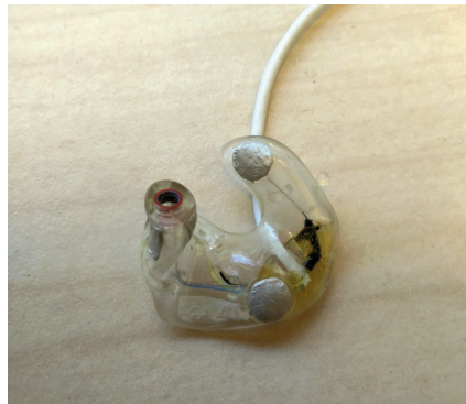
Examples of in-ear EEG mounts. ©2016 Mikkelsen.kaare, CC BY-SA 4.0, via Wikimedia Commons https://commons.wikimedia.org/wiki/File:Ear-EEG2.jpg
