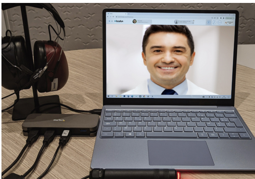
Figure 1. SHOEBOX patient side setup: headset, bone vibrator, patient response button and video-otoscope are connected to a laptop through a regular USB Hub. Software is accessible thanks to a web browser.
