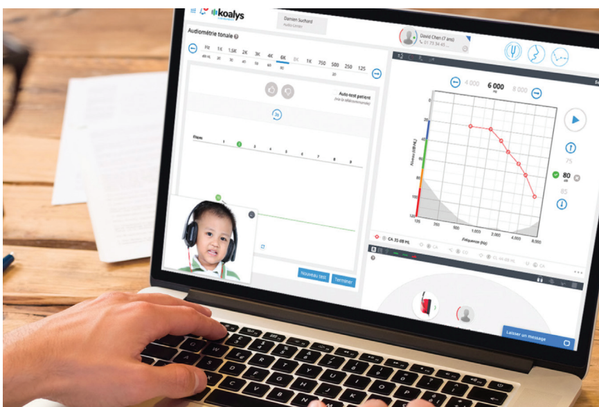
Figure 2. SHOEBOX expert side setup: any regular computer with a web browser and video conferencing capabilities (camera, microphone, speakers).
