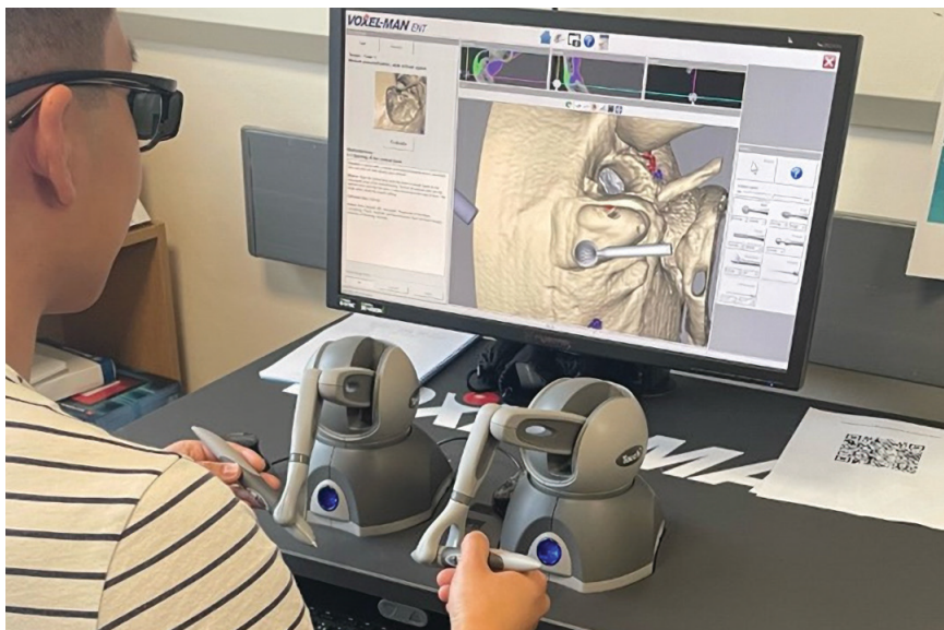
Figure 1. Digital temporal bone dissection simulator. This console is produced by VOXEL-MAN but others are available.
