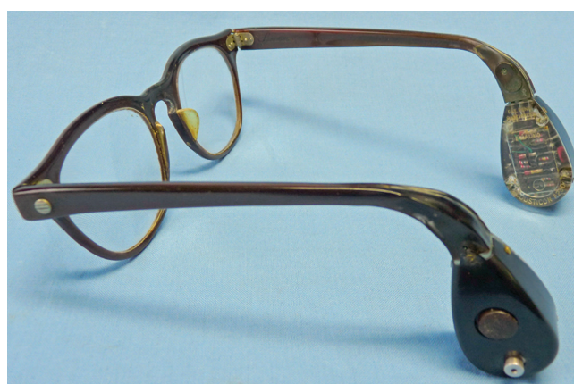
Figure 2. The Acousticon Model A-230 eyeglass hearing aid showing how the electronics were all contained in the tips of the temple pieces in this model.
