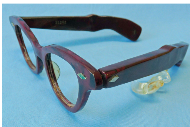
Figure 1. Otarion Model L10 'Listener' eyeglass hearing aid – the world's first transistorised eyeglass hearing aid. Note the thick, heavy temple pieces. Both were needed for this hearing aid to work.
