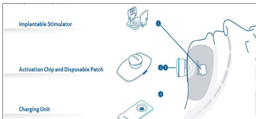
Figure 1: Schematic of Genio Nyxoah bilateral hypoglossal nerve implant components.
