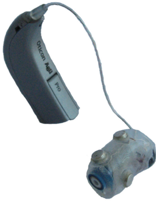
Figure 3: Research version of a hearing aid with built-in EEG function.
